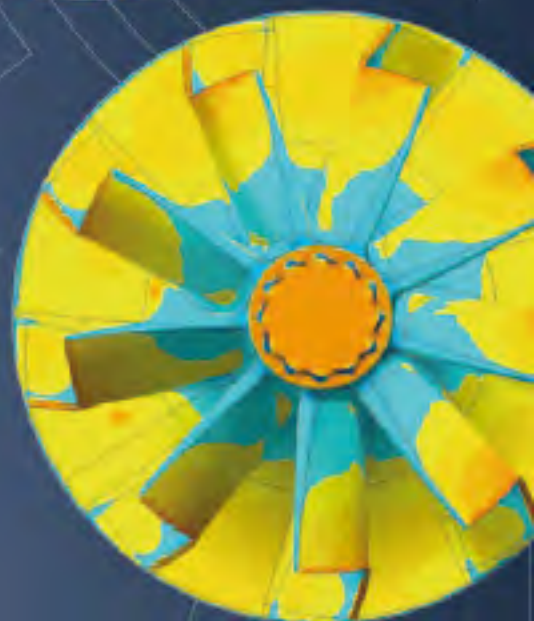
Inspection of a turbine wheel, deviations to CAD data (false colour map)
